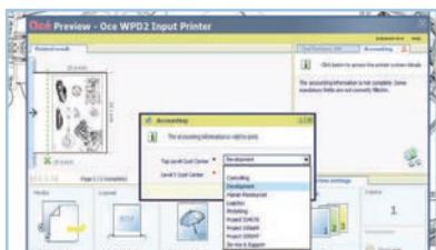
Users submit print jobs via the Windows® Printer Driver 2. They apply all appropriate settings and can select a cost center so that costs can be assigned to a department, project or customer. On pressing “print” the job is stored on the uniFLOW server, ready to be released at the device when required.
